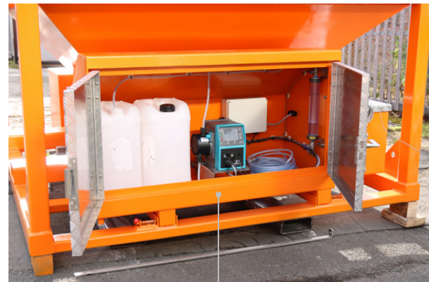
✔ Lockable cabinet housing chemical and dosing / floc pump
